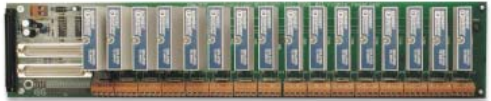
The DBK207 and DBK207/CJC accept up to 16 isolated analog input modules of any type
